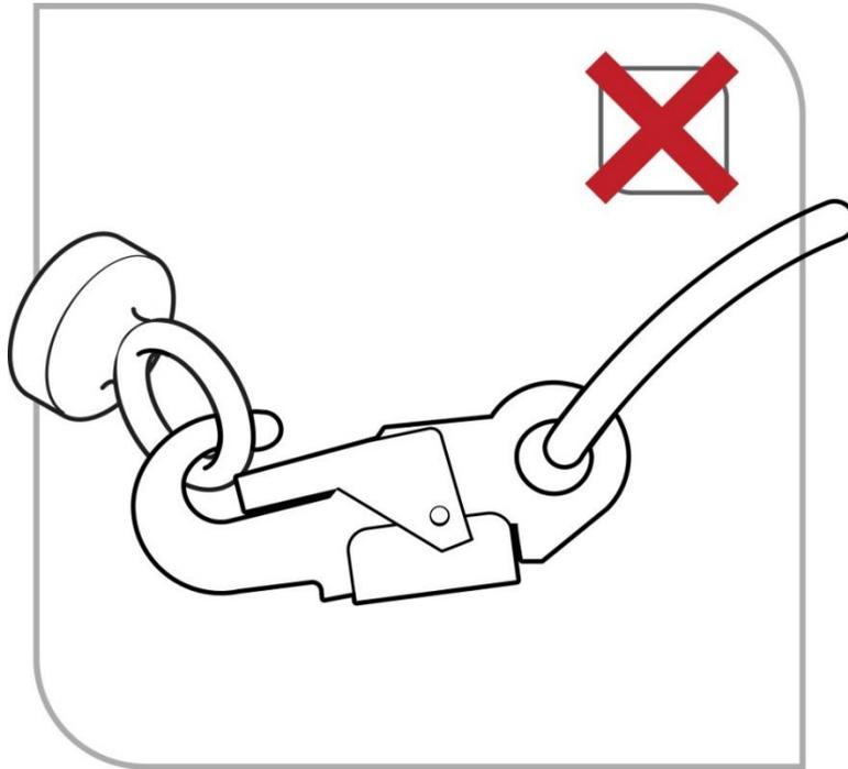
**Figure 22** Roll-out on a small diameter eyebolt
