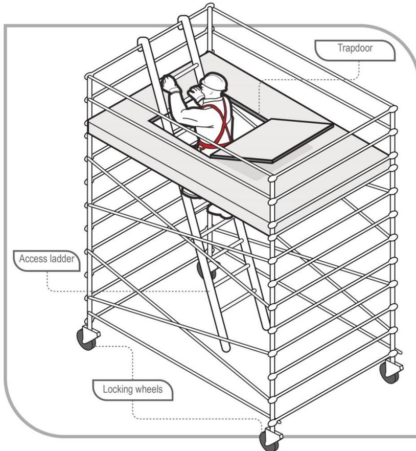
**Figure 8** Mobile scaffold with access ladder and trapdoor
