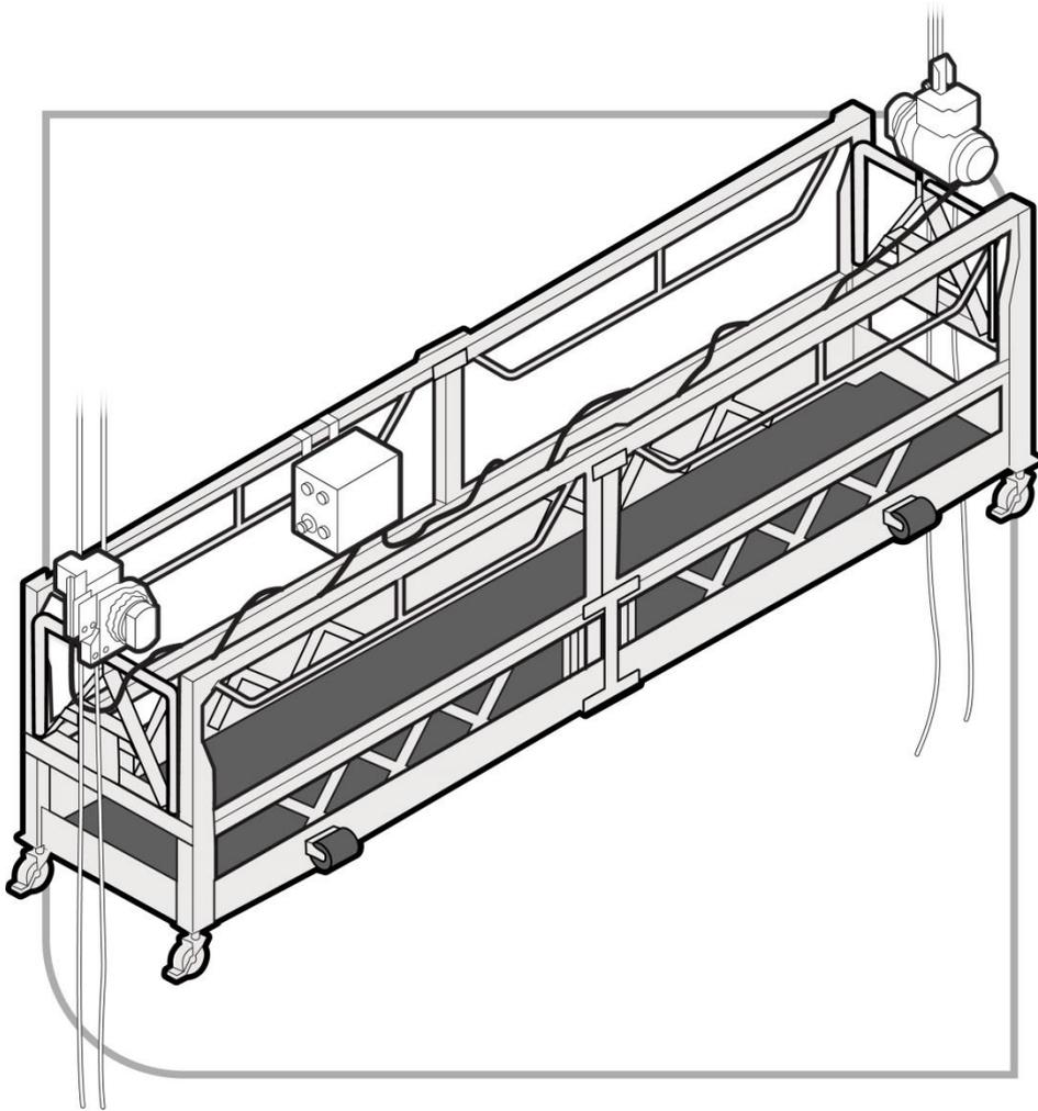
**Figure 9** Suspended (swing-stage) scaffold – cradle (suspended) end
