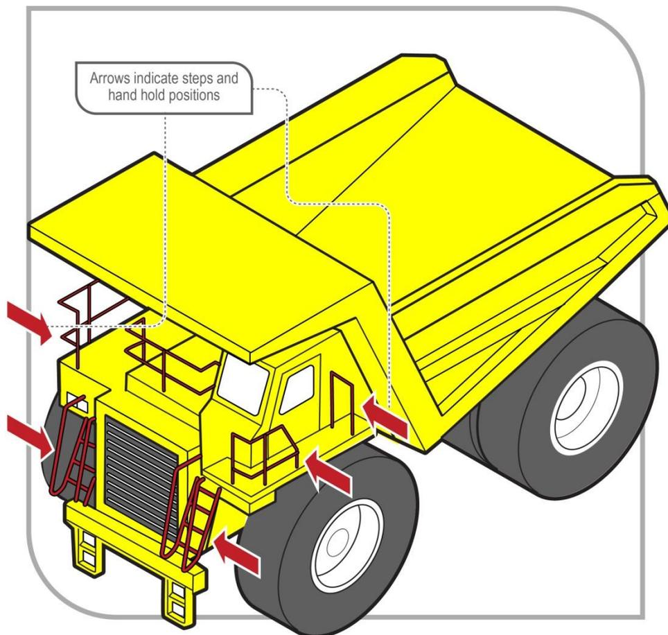
**Figure 1** Steps and handrails on dump trucks
