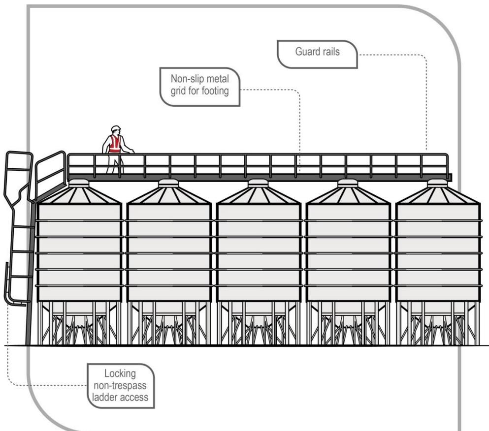
**Figure 4** Silos with platform and guard rails
