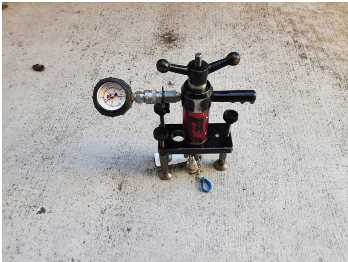
Anchor 3 pull tested at 7.5kN for 3 minutes
