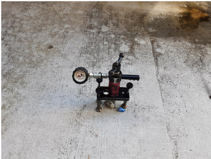
Anchor 1 pull tested at 7.5kN for 3 minutes
