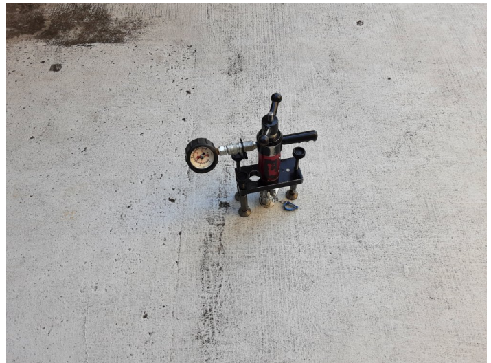
Anchor 2 pull tested at 7.5kN for 3 minutes
