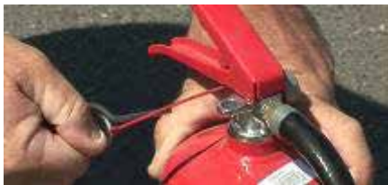
P – Pull out the safety pin
