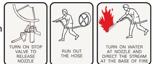
**DO NOT USE A FIRE HOSE REELS ON OR NEAR LIVE ELECTRICAL POWER**
