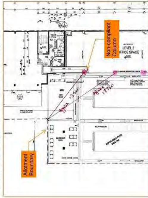
Figure 55 Location of non-compliant steel column
